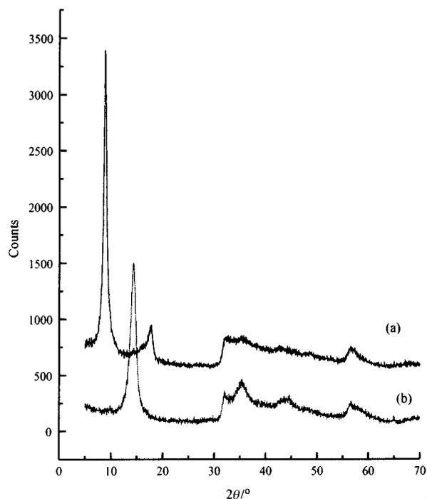
Fig. 1 Powder X-ray diffraction patterns for (a)  $(\text{C}_{10}\text{H}_8)_{0.130}(\text{H}_2\text{O})_{0.05}\text{MoS}_2$  and (b) restacked  $\text{MoS}_2$
